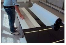
**Step 3:** Peel off the SAV so that the backing paper still lies flat on the table and the adhesive side of the SAV is facing up.
