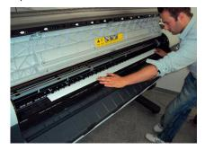
**Step 9:** Pull the material through the printer.
