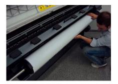
**Step 8:** Use the SAV to feed the material into the printer as usual.
