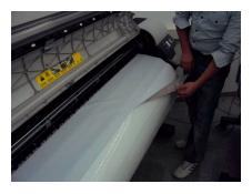
**Step 10:** Remove the SAV. fold back onto the backing paper and store for later use.
