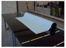
**Step 2:** Cut off a strip of SAV (self-adhesive vinyl) about 30-40cm long and about the same width as the varitex. The SAV does not have to have exactly the same size as the varitex, 2-3cm more or less do not make a difference.
