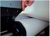
**Step 7:** Put the roll into the printer. Note: the varitex needs to be in between the SAV and the backing paper.
