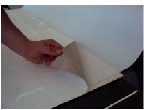
**Step 5:** Fold back the SAV to "encapsulate" the varitex between the SAV and the backing paper.
