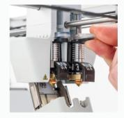
Print core AA and BB 0.25, 0.4, 0.8 mm Quick-swap nozzles for build and water-soluble support materials
