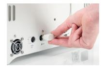
2. Connect the spool holder cable to the NFC socket and secure behind the cable clips
