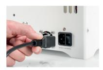
5. Connect the power cable to the printer and the other end to a power outlet
