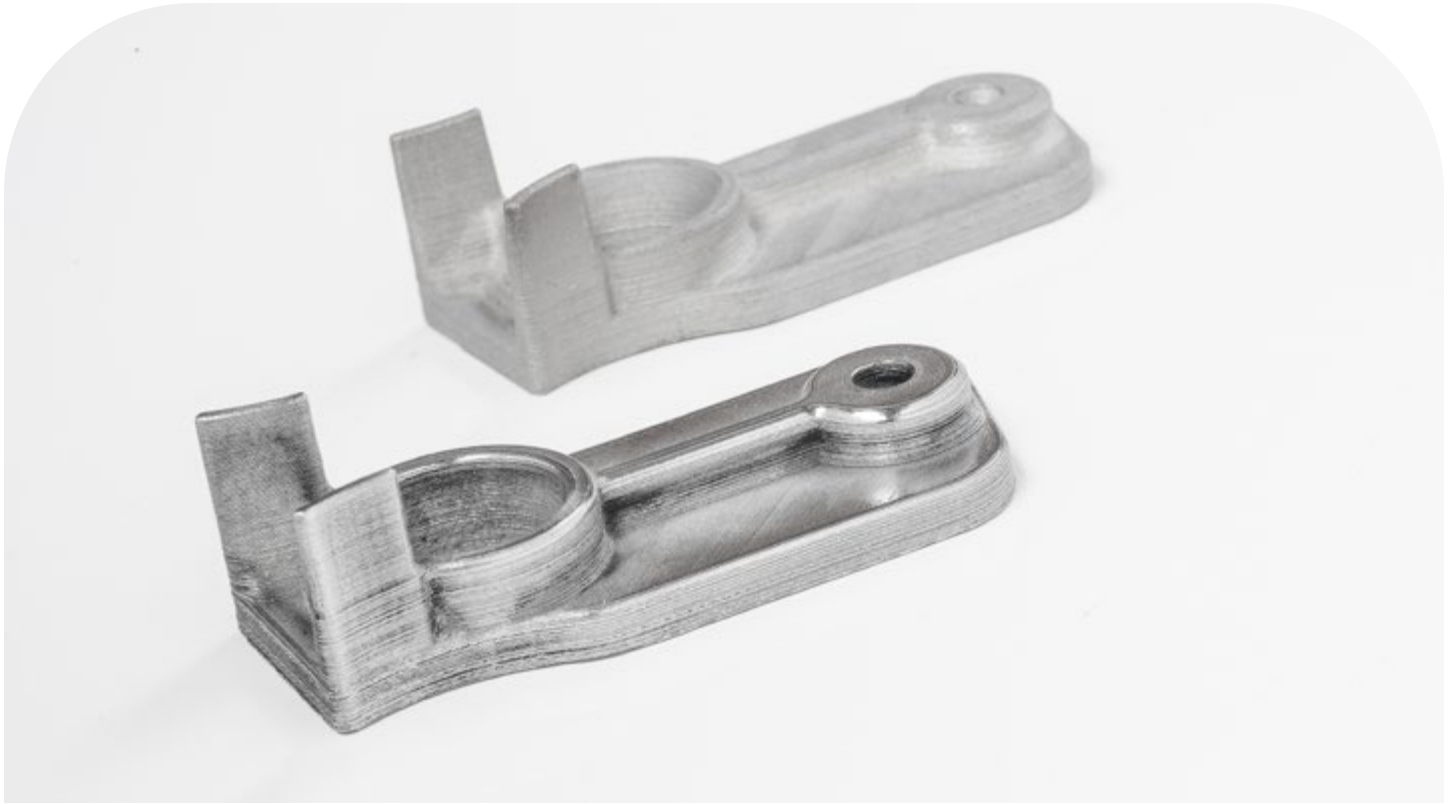
Figure 4: Before (top) and after (bottom) buffing post-processing
