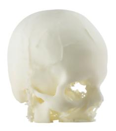
USP Class VI, which classify a material as biocompatible. <u>ABS-M30i™</u> meets these criteria so it can be used for products that come in contact with skin, food and medications.
