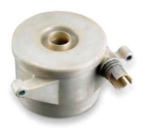
The first high-performance engineered thermoplastic available for FDM was PPSF (also called PPSU). This super material was added for under-the-hood and other advanced applications, where other plastics can succumb to heat and chemical attack. PPSF has excellent heat resistance (372 °F/189 °C heat deflection temperature) and chemical resistance. It is mechanically superior to other FDM materials outside the high-performance materials. PPSF is resistant to oils, gasoline, chemicals and acids.
