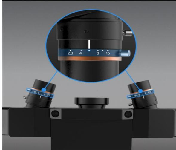
11) Lose the screw on the focal length and double-click the left and right camera windows to zoom in and check the clarity of the circle border. After the adjustment is completed, tighten the screw to prevent loosening to limit the scanning effect.
