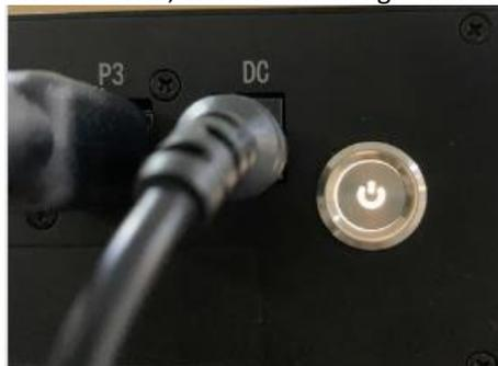
2) Press power button again to turn off the device, and the switch light turns off.
