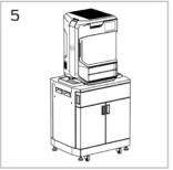
Caution: Remove the printer before moving the base station.
