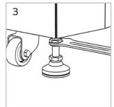
The base station should be used on a flat, stable surface. Move to the final position prior to lowering the feet.
