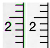
Color fringe removal (CFR) technology Color Fringe Removal (CFR) is an advanced Contex patented filtering technology designed to remove the fringes inherent in CIS strobing scanning devices.
